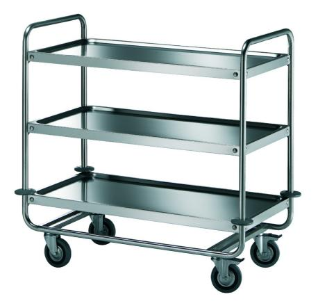
Trolley with pressed shelves, carrying frame made in stainless steel 18/10, round tube Ø 25 mm, pressed tray-shaped soundproof shelves made in sating stainless steel 18/10 with perfectly rounded upper and lower edges. 4 grey swivelling rubber wheels Ø 125 mm, rubber bumpers. Capacity 130 Kg each shelf. Three-shelves trolley mm 1100x680x1020h - 311.BC
