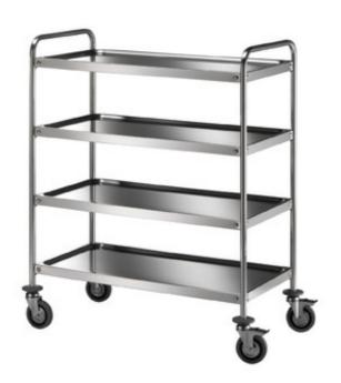
Shelves trolley made in 18/10 stainless steel, carrying frame made in 18/10 stainless steel, round tube Ø 25 mm, tray-shaped soundproof shelves made in sating 18/10 stainless steel with perfectly rounded upper and lower edges. 4 grey rubber swivelling wheels Ø 125 mm, rubber bumpers. Four-shelves trolley mm 900x580x1250h - 414.AC
