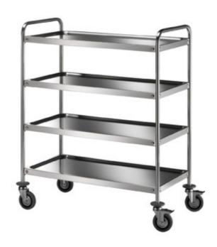
Shelves trolley made in 18/10 stainless steel, carrying frame made in 18/10 stainless steel, round tube Ø 25 mm, tray-shaped soundproof shelves made in sating 18/10 stainless steel with perfectly rounded upper and lower edges. 4 grey rubber swivelling wheels Ø 125 mm, rubber bumpers. Four-shelves trolley mm 1100x580x1250h - 414.A
