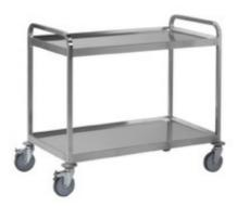
Trolley for heavy transport, capacity 500 Kg, welded carrying frame made in stainless steel 18/10, square tube 25x25 mm, bended and reinforced shelves, welded to the frame. 4 grey rubber swivelling wheels Ø 150 mm, rubber bumpers. Three-shelves trolley mm 1060x610x950h - 408.AC
