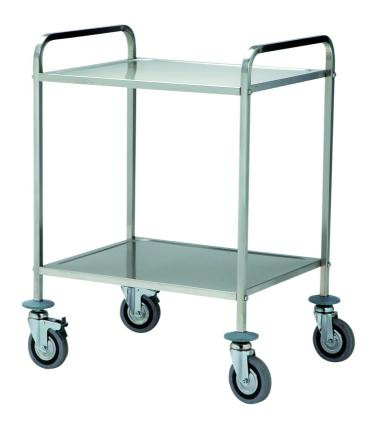
Shelves trolley made in 18/10 stainless steel, carrying frame made in 18/10 stainless steel, square tube 20x20 mm bended shelves h 20 mm, 4 grey rubber swivelling wheels 125 mm, rubber bumpers. Two-shelves trolley mm 600x560x900h - 201.AC
