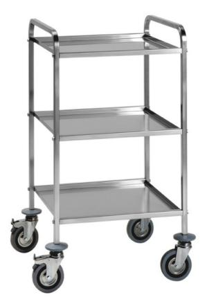
Shelves trolley made in 18/10 stainless steel, carrying frame made in 18/10 stainless steel, square tube 20x20 mm bended shelves h 20 mm, 4 grey rubber swivelling wheels 125 mm, rubber bumpers. Three-shelves trolley mm 900x560x1020h - 304.AC
