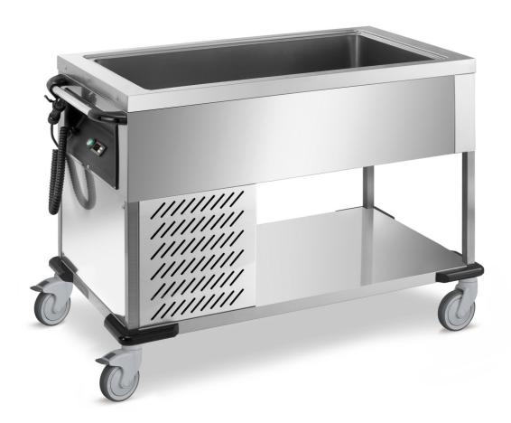
Refrigerated trolley (GN not included). Carrying frame made in stainless steel 304 AISI 18/10. Pressed no-drops basin h 200 mm. Temperature controlled by a digital thermostat; refrigerating system, consisting of HP 1/8 500 W - 230 V 50/60Hz. Spiral cable with CE plug and socket hoot. Push handle. 4 grey rubber swivelling wheels Ø 125 mm not marking, 4 bumpers made in black PVC. Refrigerated trolley, capacity 4 GN1/1 h 200 mm, mm 1500x640x900 h - 0131.AD
