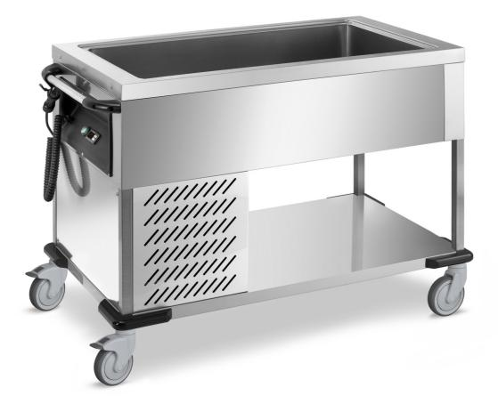
Refrigerated trolley (GN not included). Carrying frame made in stainless steel 304 AISI 18/10. Pressed no-drops basin h 200 mm. Temperature controlled by a digital thermostat; refrigerating system, consisting of HP 1/8 500 W - 230 V 50/60Hz. Spiral cable with CE plug and socket hoot. Push handle. 4 grey rubber swivelling wheels Ø 125 mm not marking, 4 bumpers made in black PVC. Refrigerated trolley, capacity 3 GN1/1 h 200 mm, mm 1200x640x900 h - 0131.A
