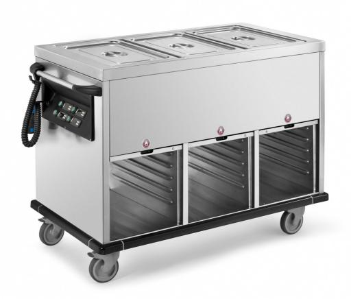
Heated bain-marie trolley unique basin, structure completely made in stainless steel 18/10 AISI 304, dry/bainmarie heating, temperature controlled by digital thermostat 30° - 90° C°. Printed unique basin with rounded corners, for 3 GN1/1 h 200, anti-drop board, insulated double wall, spiral electrical wire with CE plug and hooker for the plug, ergonomic push handle. Under compartments with hiding tilting doors, with 5 printed slideways, pitch 55mm, capacity 2 GN1/1 h 100 mm + 1
