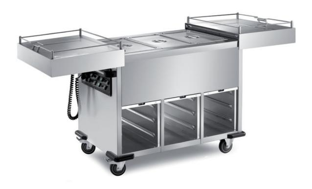
Heated bain-marie trolley separated basins (GN not included), structure completely made in stainless steel 18/10 AISI 304. Dry/bainmarie heating, temperature controlled by digital thermostat 30° - 90° C° 230 V 50/60 Hz. Deep-drawn separated basins with rounded corners, for 3 GN1/1 H 200, anti-drop board, insulated double wall, spiral electrical wire with CE plug and hooker for the plug, ergonomic push handle, Under compartments with hiding tilting doors, with 5 deep-drawn slideways,
