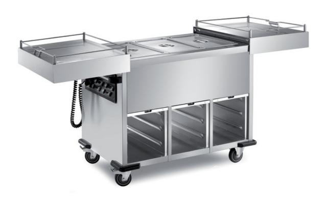
Heated bain-marie trolley separated basins (GN not included), structure completely made in stainless steel 18/10 AISI 304. Dry/bainmarie heating, temperature controlled by digital thermostat 30° - 90° C° 230 V 50/60 Hz. Deep-drawn separated basins with rounded corners, for 2 GN1/1 H 200, anti-drop board, insulated double wall, spiral electrical wire with CE plug and hooker for the plug, ergonomic push handle, Under compartments with hiding tilting doors, with 5 deep-drawn slideways,
