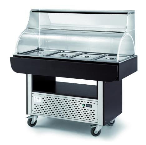
Wall refrigerated display cabinet, wengé colour (GN not included) stainless steel structure with wengé panels. Pressed bowl with antidrop border. Plexiglas superstructure with semicylindric dome. Hermetic refrigerating system HP 1/8 500W 230V 50/60Hz single-phase. Digital temperature control 0°-15°C. 4 wheels, Ø 125 mm, 2 of which with brakes. Capacity 3GN 1/1 h 150. Capacity 3 GN 1/1 h 200 mm - 500 W; dim. mm 1100x640x1400 h - 714.P
