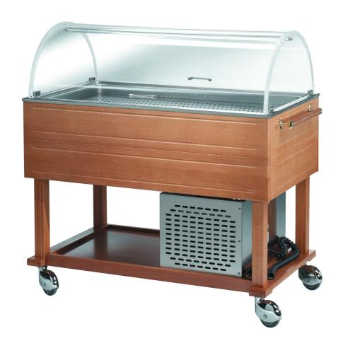
Refrigerated trolley (GN not included), Carrying frame and shelves made in solid wood. Pressed no-drops basin made in stainless steel 18/10 AISI 304. Dome made in transparent plexiglass. Hermetic circuit refrigerating system, consisting of HP 1/8 500 W - 230 V, single-phase compressor unit. The temperature is controlled by a digital thermostat approx. -5°+10° C. 4 swivelling wheels covered with casing Ø 100 mm. Refrigerated trolley, semi-cylindrical dome, capacity 3 GN 1/1 h 200 mm
