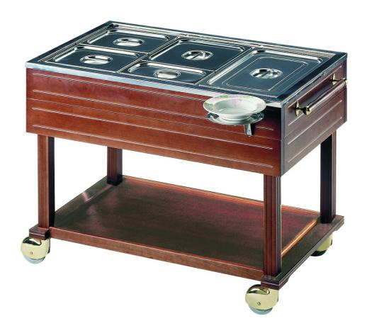
Heated trolley made in wood (GN not included), carrying frame made in solid wood. Pressed basin no-drops with double isolated wall with drilled grill. Electric water-bath heating 2000W - 230V. Temperature controlled by a digital thermostat 30°-90°C. 4 swivelling wheels with brass plated cap Ø 100 mm. Heated trolley 2000 W, capacity 3 GN 1/1 h 150 mm (50-60 meals). Dim. mm 1200x640x900 h - 025.LM
