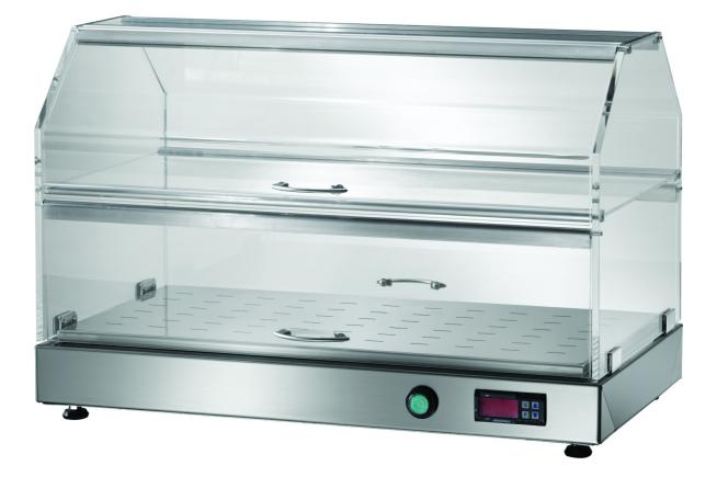
Heated display cabinets (one shelf), base made in stainless steel 18/10 AISI 304, upper structure made in transparent plexiglass. One intermediate shelf. Thermostat 30°- 90° C. Heating 230 V. Heated display cabinet (1 shelf) 210 W, dim. mm 630x350x530 h - VT2
