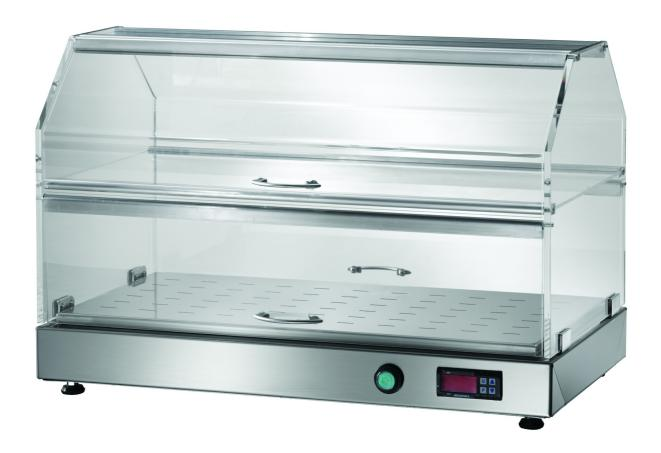
Heated display cabinets (one shelf), base made in stainless steel 18/10 AISI 304, upper structure made in transparent plexiglass. One intermediate shelf. Thermostat 30°- 90° C. Heating 230 V. Heated display cabinet (1 shelf) 180 W, dim. mm 530x350x530 h - VT1
