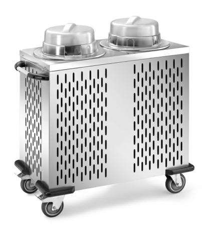
Refrigerable dishes distributor with 2 adjustable columns. Entirely made in 18/10 stainless steel with 2 fixed wheels and 2 swivelling with brake diam. 125 mm and corner bumper. Lids included. Capacity 100-120 dishes, diam 28/32 Dim. mm 1030x530x1060 h - CSG/2F
