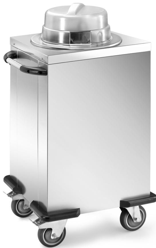
Dishes distributor with 1 fixed column. Entirely made in 18/10 stainless steel with 2 fixed wheels and 2 swivelling with brake diam. 125 mm and corner bumper. Lids included. Capacity 50-60 dishes, diam 16/21, dim mm 510x480x1060 h - CSL/1N
