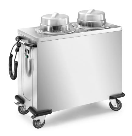
Heated dishes distributor with 2 adjustable columns. Entirely made in 18/10 stainless steel with 2 fixed wheels and 2 swivelling with brake diam. 125 mm and corner bumper. Lids included. Digital thermostatic regulation +30° - +90°C, 900 W - 230 V 50/60 Hz. Capacity 100-120 dishes. diam 18/28. Dim. mm 1030x480x1060 h - CSP/2C
