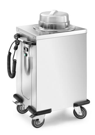
Heated dishes distributor with 1 adjustable column. Entirely made in 18/10 stainless steel with 2 fixed wheels and 2 swivelling diam. 125 mm with brake and corner bumper. Digital thermostatic regulation +30° - +90°C, 0.9 kW - 230 V 50/60 Hz. Lids included. Capacity 50-60 dishes, diam 18/28, 900 W. Dim. mm 600x480x1060 h - CSP/1C
