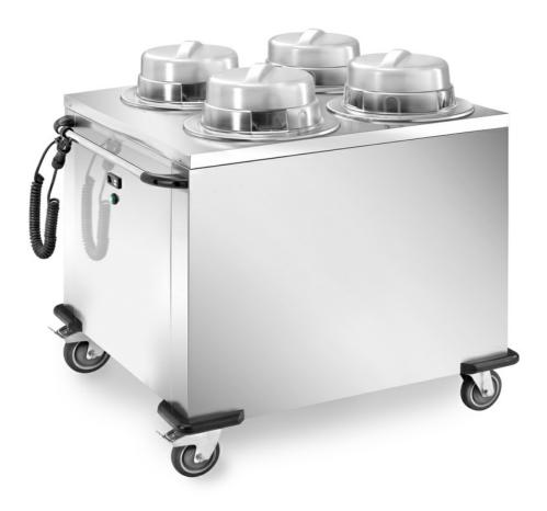
Heated dishes distributor with 4 adjustable columns. Entirely made in 18/10 stainless steel with 2 fixed wheels and 2 swivelling with brake diam. 125 mm and corner bumper. Lids included. Digital thermostatic regulation +30° - +90°C, 2000 W - 230 V 50/60 Hz. Capacity 200-240 dishes, diam 28/32 Dim. mm 1130x990x1060 h - CSG/4C
