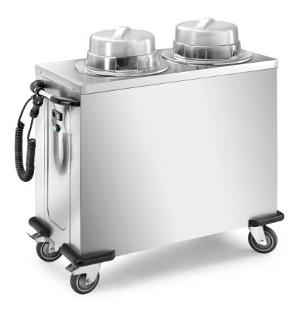
Heated dishes distributor with 2 adjustable columns. Entirely made in 18/10 stainless steel with 2 fixed wheels and 2 swivelling with brake diam. 125 mm and corner bumper. Lids included. Digital thermostatic regulation +30° - +90°C, 900 W - 230 V 50/60 Hz. Capacity 100-120 dishes, diam 28/32. Dim. mm 1130x530x1060 h - CSG/2C
