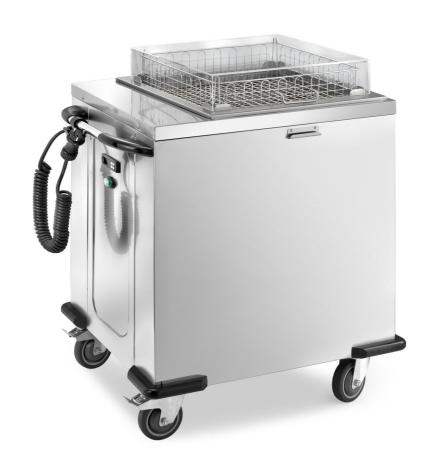
Heated basket elevator with 1 column. Entirely made in 18/10 stainless steel with 2 fixed wheels and 2 swivelling with brake Ø 125 mm and corner bumper. Lids included. Digital thermostatic regulation +30° - +90°C, 2000 W - 230 V 50/60 Hz, 900 W. Capacity basket 6, dim mm 500x500x115 h or capacity basket 9, dim mm 500x500x75 h - CSC5/5
