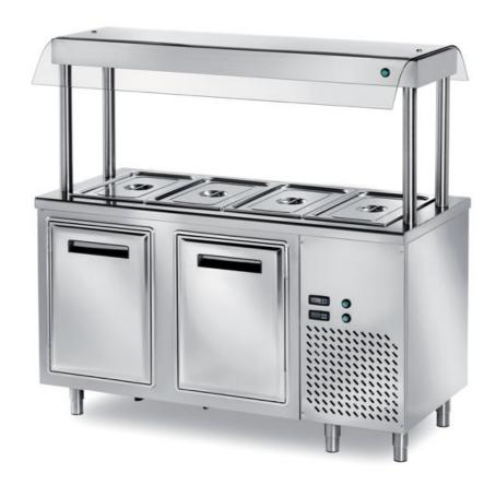
Refrigerated central island for salads and hors-d'oevres with a h 200 bowl. Refrigerated doors + motor compartment with 2 controls. Upper shelf equipped with curved glass and with internal lighting. GN containers not included, mm 1500x700x1500h - TIN/15
