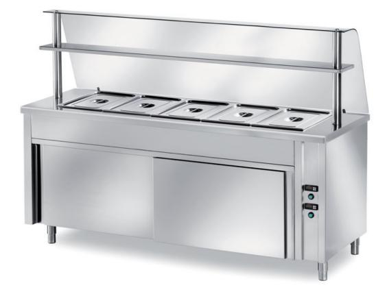
Self service heated table, heated and ventilated lower cabinet, 4000 Watt, bainmarie half-rounded bowl H200, capacity 3 bowl GN 1/1 h 150 (GN not included) mm 1200x700x1400 h + curved toughened glass -SFC/12
