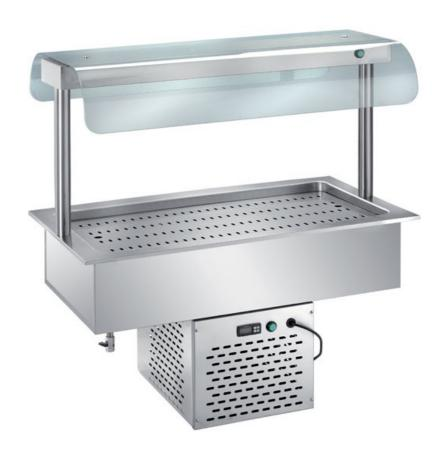
Static refrigerated drop-in basin mm.200h, temperature -2�/+15�C, with upper toughened glass with lights, dim. mm.1110x640x820h - 212W - cap. 3GN1/1 h 200 - 120.TN
