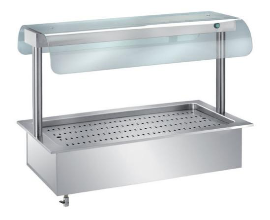
Bain-marie drop-in basin mm.200h, temperature 0�/+90�C, with upper toughened glass with lights, dim. mm.1850x640x820h - 1800W - cap. 5GN1/1 h 200 - 180.TB
