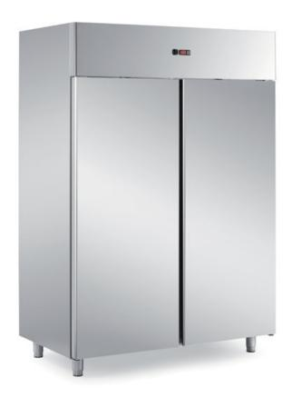
Refrigerated cabinet TN in stainless steel AISI 304 18/10, Lt. 1400, insulation thickness 75 mm with 3 plastic grids mm. 530x650, automatic defrosting and condensation evaporation, digital control. Lighting and keys included, Temp. -2/+10°C dim. mm 1480x800x2050 h - GS500
