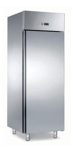
Refrigerated cabinet TN with 1 door, Lt. 700 temperature -2°/+8° C, lighting and keys included, dim. mm 740x830x2010 h insulation thickness 60 mm with 3 plastic grids mm. 530x650, automatic defrosting and condensation evaporation, digital control. - GT250
