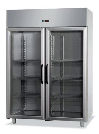
Refrigerated cabinet TN in stainless steel AISI 304 18/10, Lt. 1400, insulation thickness 75 mm with 3 plastic grids mm. 530x650, automatic defrosting and condensation evaporation, digital control. Glass doors. Temp. -2/+10°C dim. mm 1420x800x2050 h - GV500
