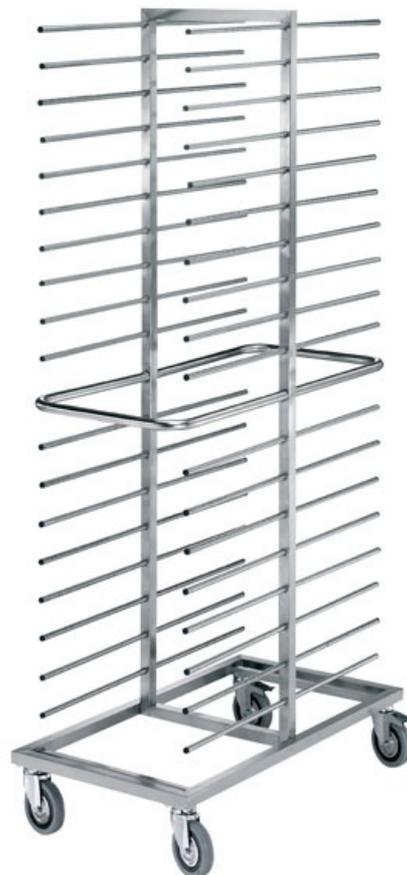
Trolley for baking tin. Welded frame made in stainless steel 18/10 AISI 304, square tube 30x30 mm. Rounded handle. 4 swivelling wheels Ø 125 mm. Capacity 32 baking tins 600x400 mm, distance between guides 95 mm; dim. mm 960x500x1760 h - 641.A
