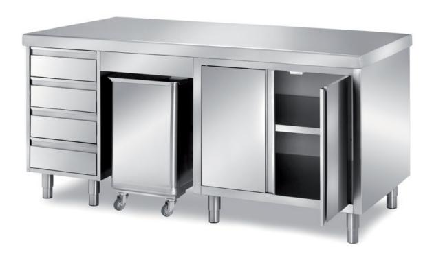
Central bakery table composition n°1, top H=60mm rounded front and back edge, n°1 set of 4 drawers + ingredient bin CPD/1 + pass through element with swing doors mm 2000x800x850 h - TVC/A
