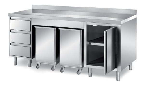
Cabinet table with I swing door, with 2 ingredient bins on wheels and a set of 3 drawers H=150mm, with backsplash dim. mm 2000x800x850 hr TVC28/20A
