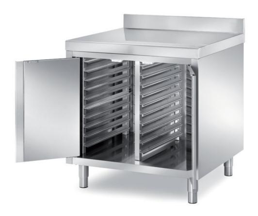
Cabinet table with 2 swing doors and 2 pans rack compartments cm 40x60 - top with rounded front edge h 6 cm - dim. mm 1000x800x850 h - TPG28/10
