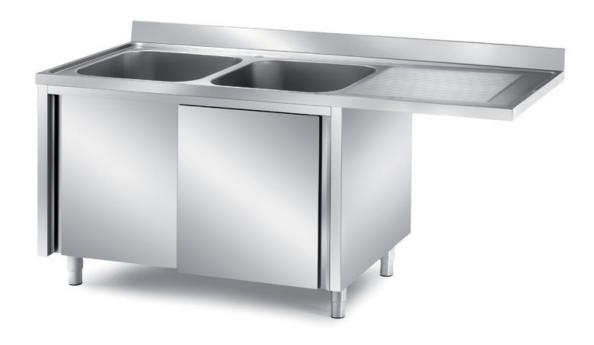
Cabinet sink with swing doors with overhanging top for dishwasher installation - with 1 bowl mm 500x500x300 h and 1 LH drainboard mm1300x700x850h - LLS1/13
