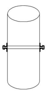
Flange for joint round ducts "tiposistem" diam. 60 STAINLESS STEEL -
