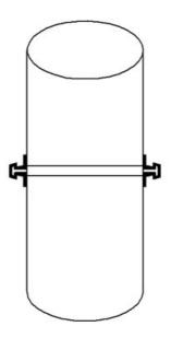
Flange for joint round ducts "tiposistem" diam. 50 STAINLESS STEEL - FLT50INOX
