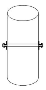
Flange for joint round ducts "tiposistem" diam. 20 STAINLESS STEEL -
