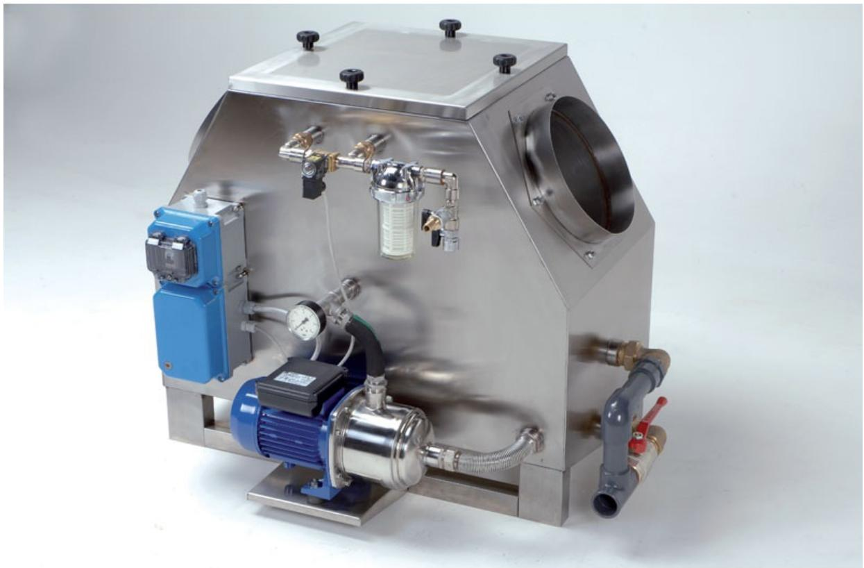
Blast soot, automatic operation, smoke treatment by water system and filtration by micro net filters G2 755. Cap. 1500/3500 mc/h - AGF/350
